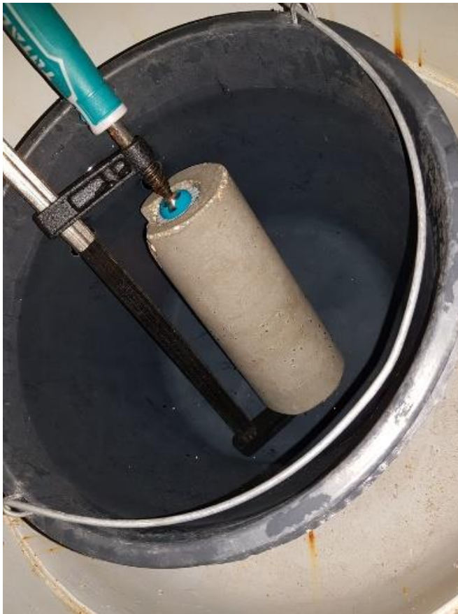
Figure 2.1 - UUT during Immersion Test
